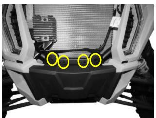
• Locate the mounting plate toward the bottom of the radiator
