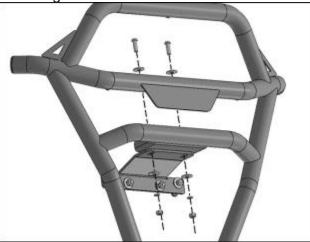
• From behind the lower mounting plate on the vehicle, insert the Spacer Plate and the Double Bolt Plate. Attach the bottom of the Bumper to the Double Nut Plate with (2) 10mm Hex Bolts, (2) 10mm Lock Washers and (2) 10mm Flat Washers. Do not tighten hardware. **Note:** for models equipped with a tow hook, attach the tow hook to the bottom of the bumper between the Flat Washers and the bottom of the Bumper.
