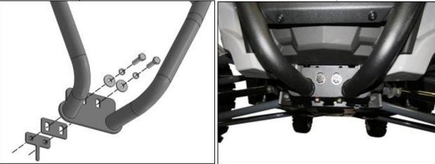
• Level and adjust the bumper and tighten all hardware.
